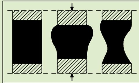
With plastic waterproofing materials it is easy to create a bond to diverse substrates. Plastic sealing compounds can be used in closed joint designs such as in pipe penetrations (see page 14).
