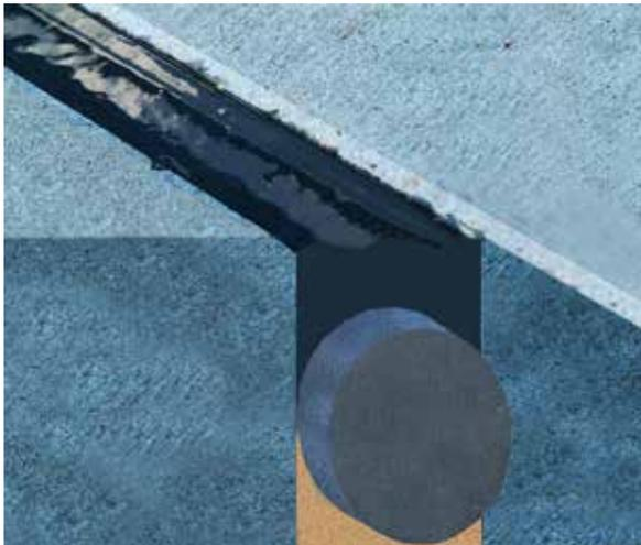
Joints connect building parts and elements that are made from different materials, enable movement and settling of the construction, and contribute to the acoustic insulation of a building. Construction joints are found in new construction, in precast construction and existing buildings. Joints must be properly planned and installed with respect to thermal transmission and air tightness so that they do not become a weak point in the building.
