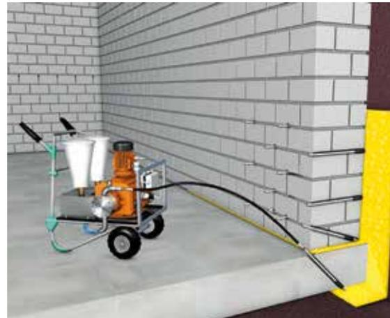
*In cases where an existing basement is leaking and the soil surrounding the building cannot be excavated, the waterproofing has to be done from the inside. With KÖSTER PUR Gel it is possible to create an exterior waterproofing layer*
