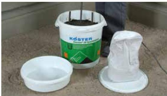
The KÖSTER Deuxan® 2C bucket has an insert which contains a bag with the powder component. The powder component is slowly mixed into the bitumen component using a slow rotating stirring device. Mixing time is 3 minutes.
